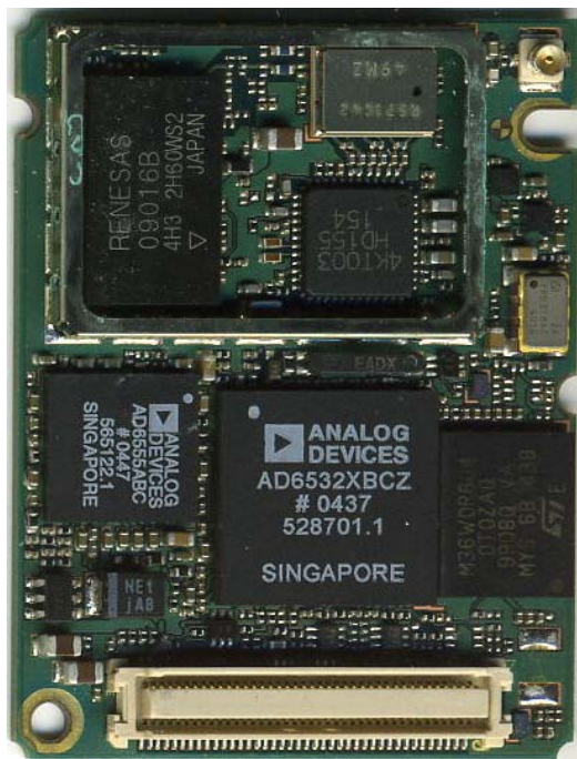
TC65: component side shielding opened
