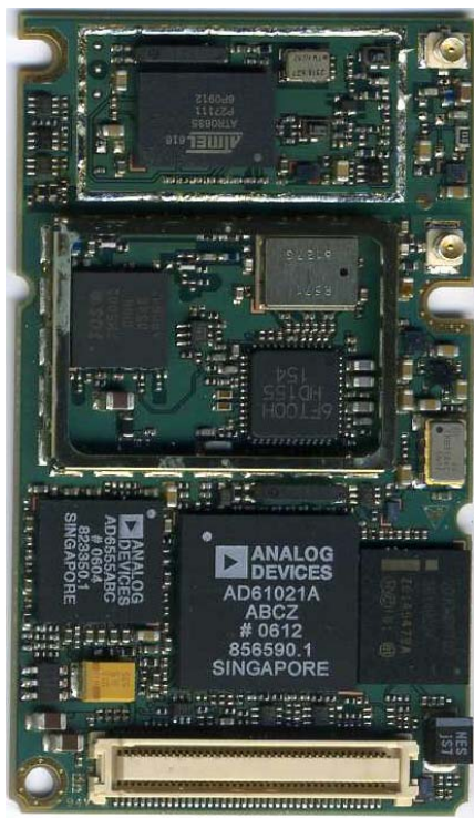
Siemens Cellular Engine XT75 / XT65 Top side without shielding
