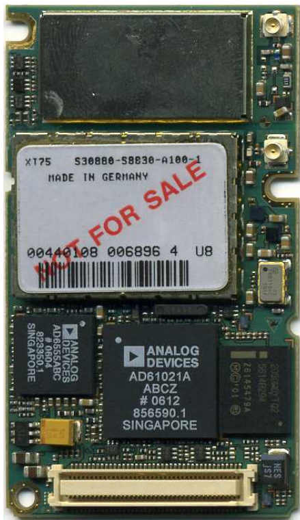
Siemens Cellular Engine XT75 / XT65 Top side
