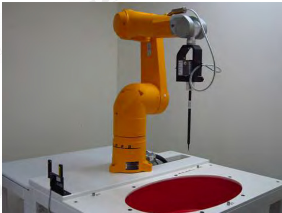
Fig.1 Photograph of the SAR measurement system
