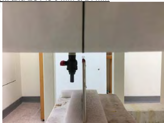
Fig.9 EUT Top side (14mm) to flat phantom
