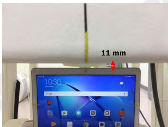
Fig.8 EUT Top side (11mm) to flat phantom
