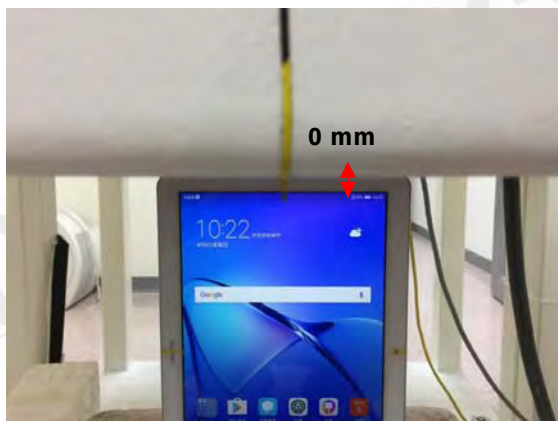
Fig.10 EUT Left side to flat phantom
