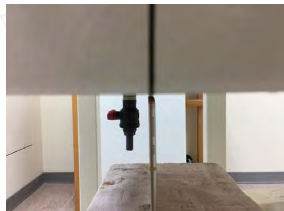
Fig.7 EUT Top side to flat phantom
