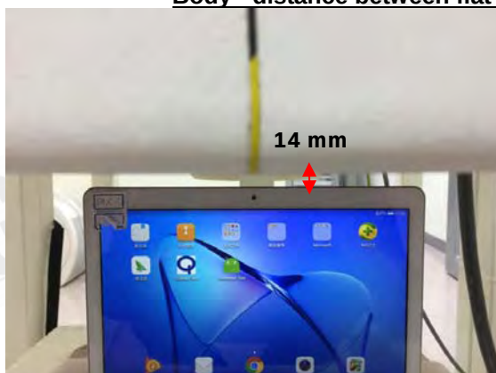
Fig.9 EUT Top side (14mm) to flat phantom
