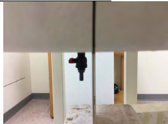
Fig.6 EUT Right side to flat phantom
