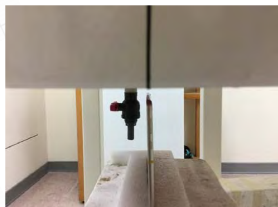
Fig.8 EUT Top side (11mm) to flat phantom
