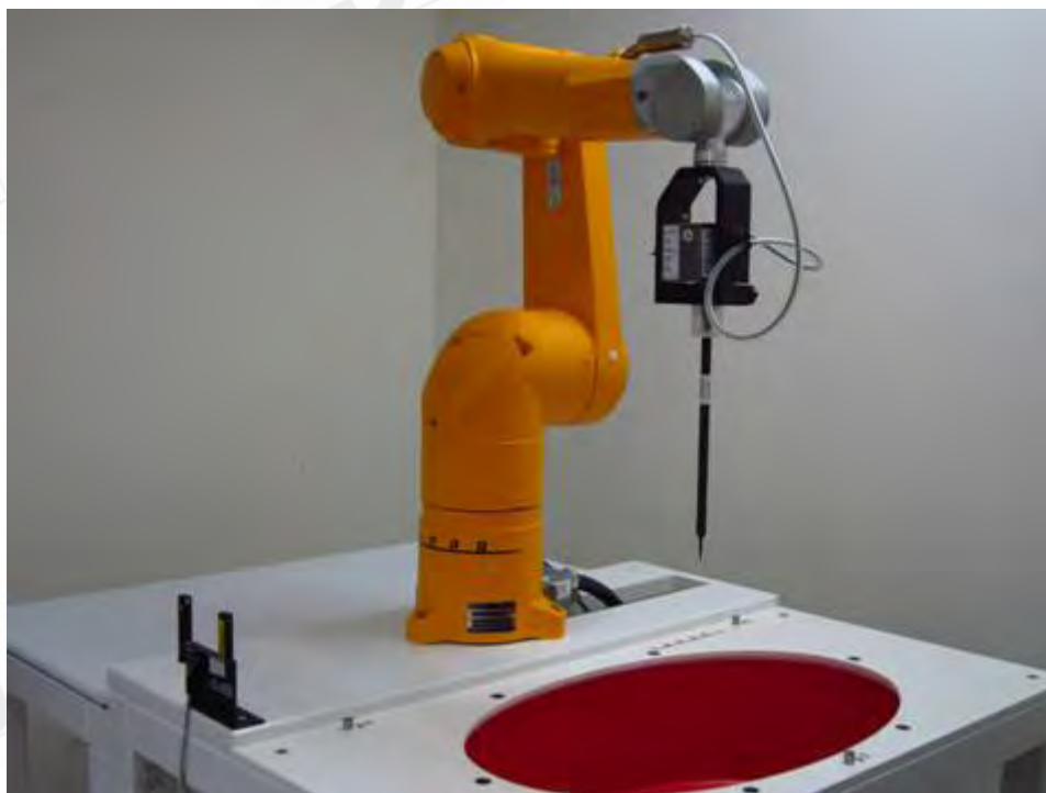
Fig.1 Photograph of the SAR measurement system
