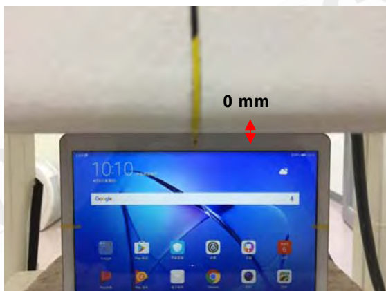
Fig.7 EUT Top side to flat phantom
