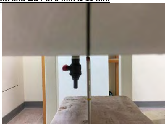
Fig.6 EUT Top side to flat phantom
