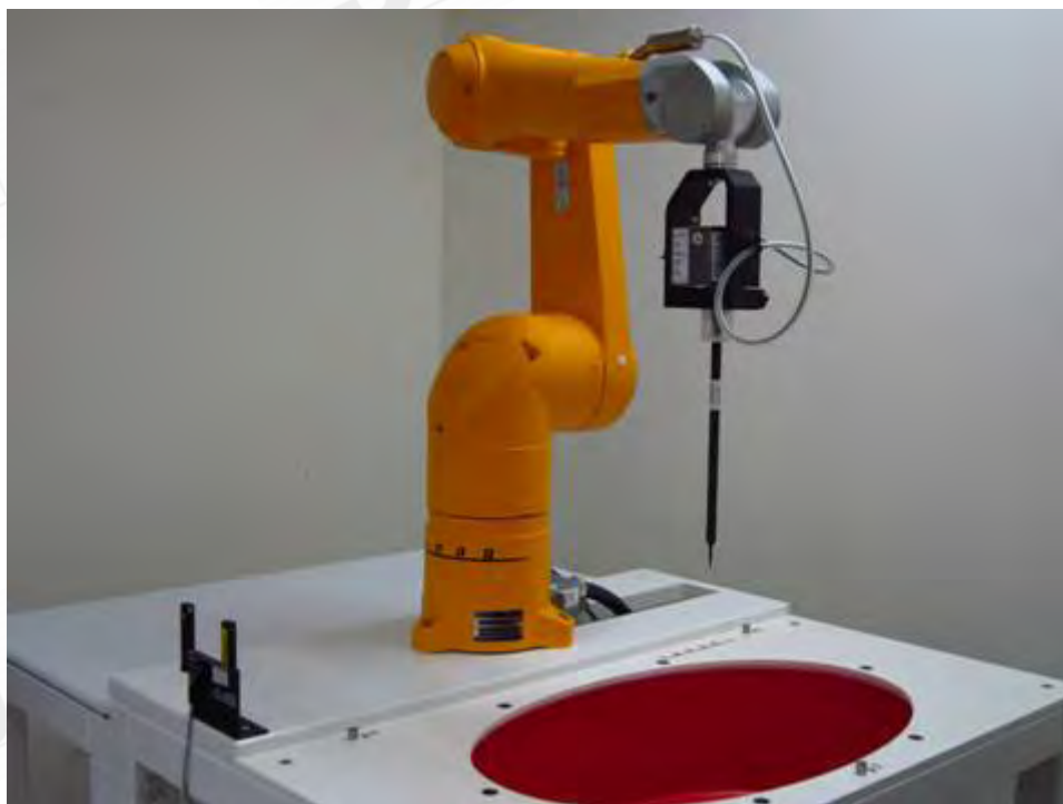
Fig.1 Photograph of the SAR measurement system
