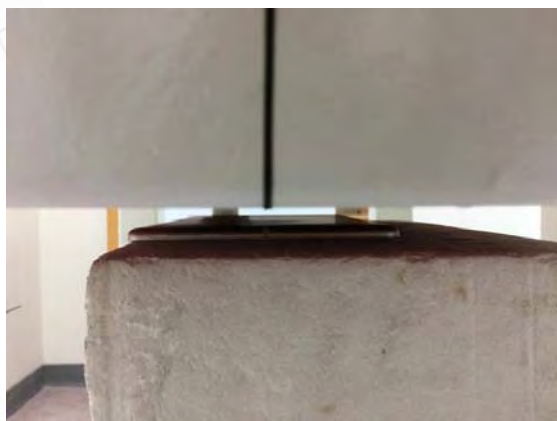
Fig.4 EUT Back side (10mm) to flat phantom
