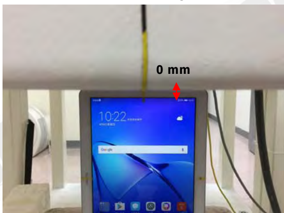
Fig.5 EUT Left side to flat phantom
