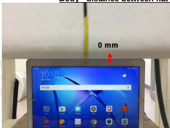
Fig.6 EUT Top side to flat phantom
