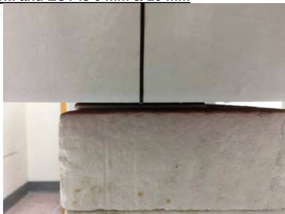
Fig.3 EUT Back side to flat phantom
