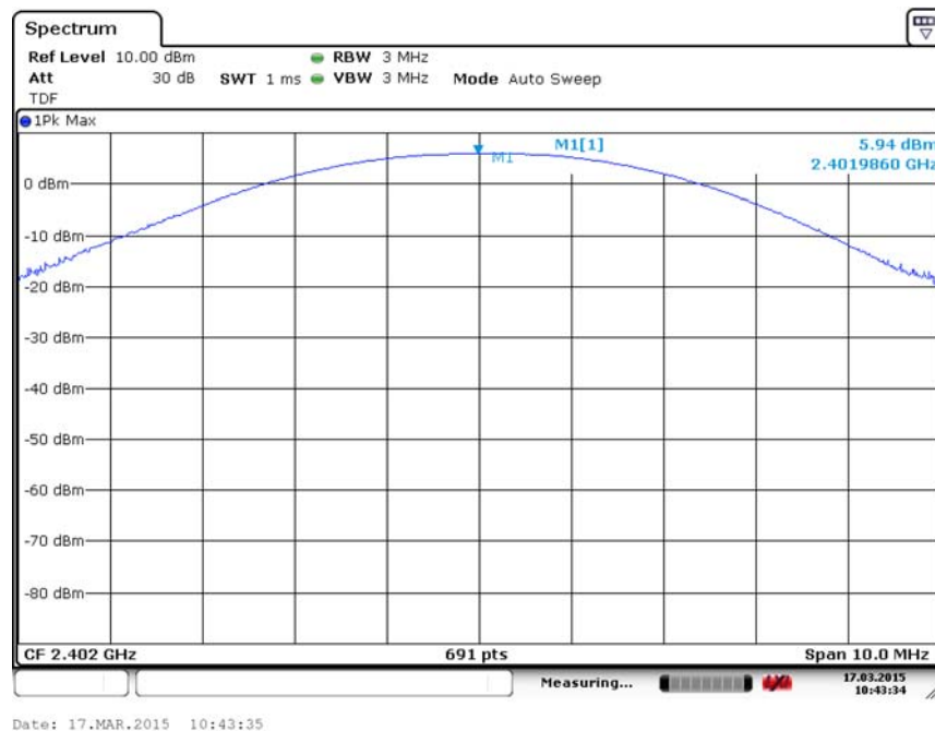
Fig.1 Maximum Peak Output Power(GFSK, Ch 0)
