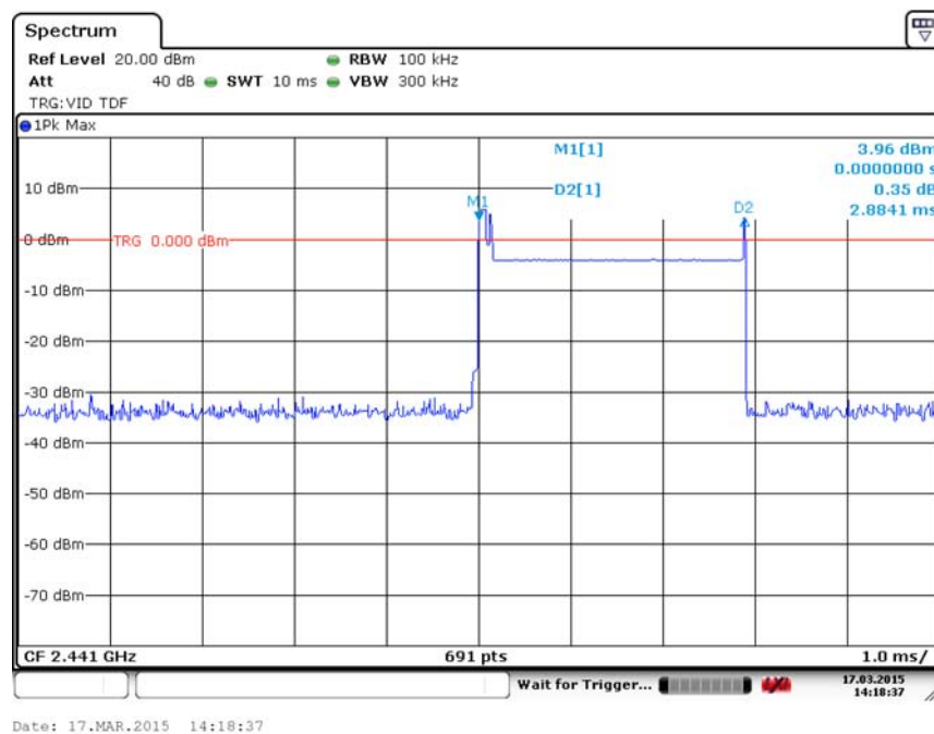
Fig. 96 Time of Occupancy(Dwell Time) (8DPSK, Ch39)
