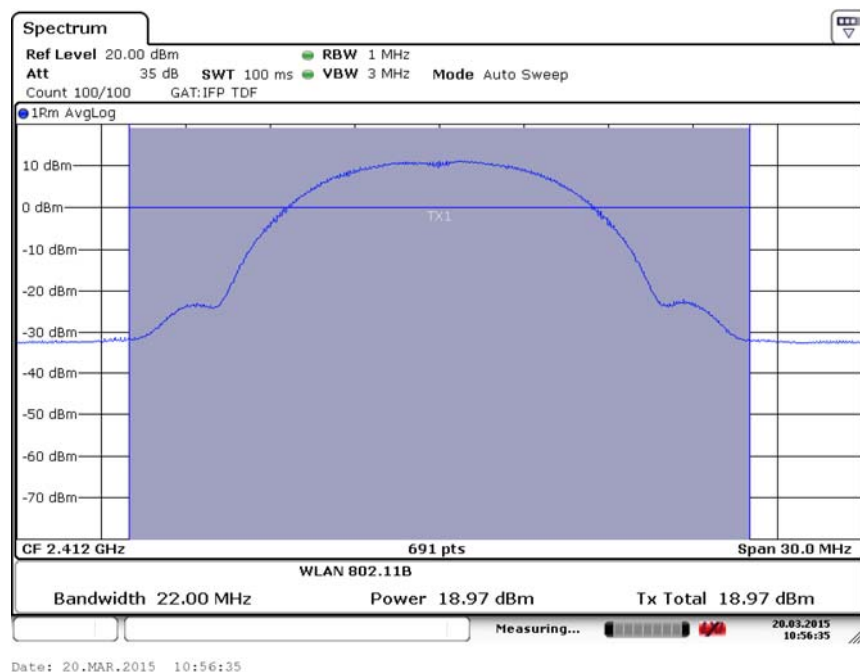
Fig.10 Maximum Average Output Power (802.11b, Ch 1,11Mbps)
