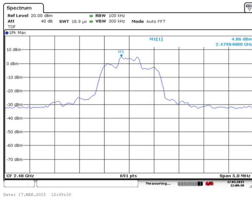
Fig. 46 Conducted Spurious Emission (8DPSK, Ch78, 2.480GHz)
