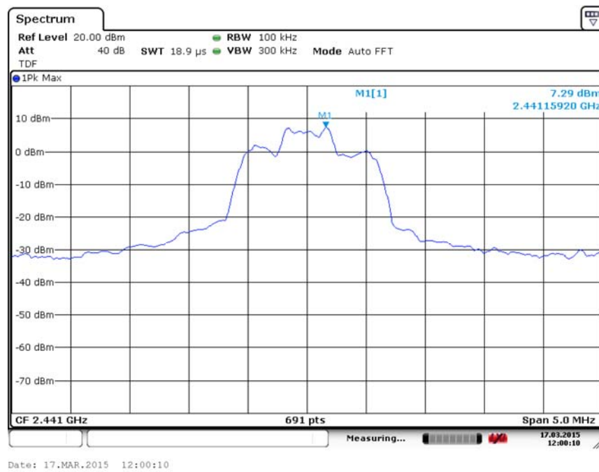
Fig. 43 Conducted Spurious Emission (8DPSK, Ch39, 2.441GHz)
