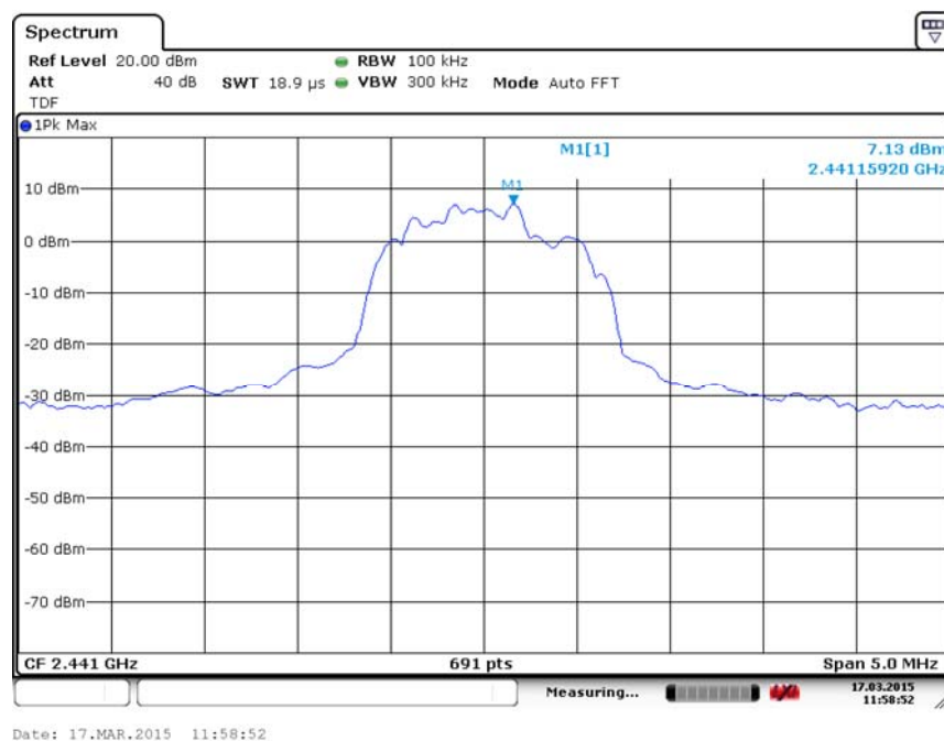
Fig. 34 Conducted Spurious Emission ( \pi/4 DQPSK, Ch39, 2.441GHz)
