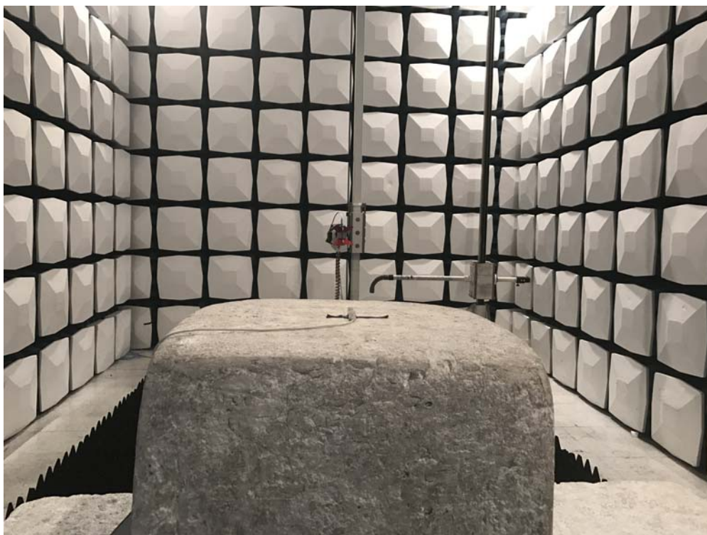
Description: Radiated Emission Test Setup for 1~18GHz
