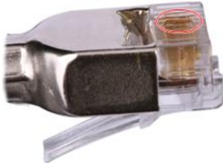
Figure 5-34 Unparallel contact strips of different heights
