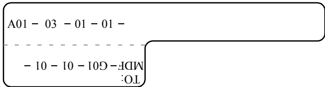
Figure 5-92 Example of labels for user cables
