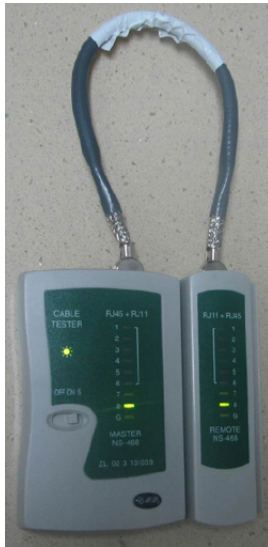
Figure 5-39 Testing the conduction and connections of wires
