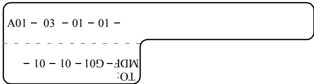
Figure 5-92 Example of labels for user cables
