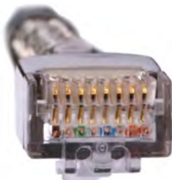
Figure 5-33 Contact strips of the same height
