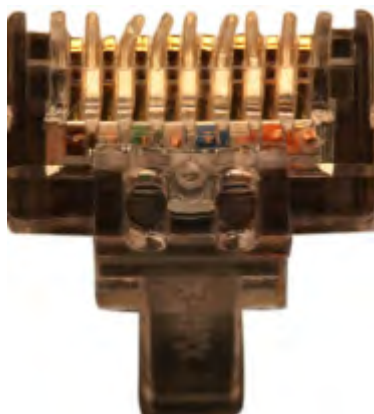
Figure 5-36 Skew plastic separators
