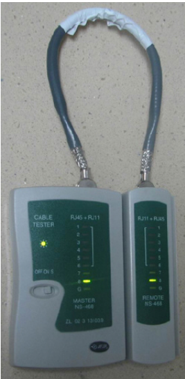
Figure 5-39 Testing the conduction and connections of wires
