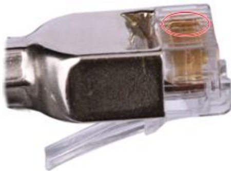
Figure 5-34 Unparallel contact strips of different heights
