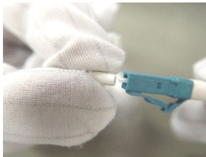
Figure 5-99 Installing a protective cap on a fiber
