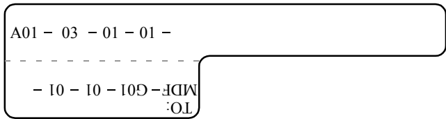
Figure 5-92 Sample label on a user cable
