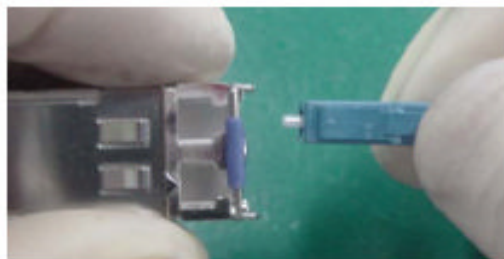
Figure 5-98 Using fibers to protect an optical module
