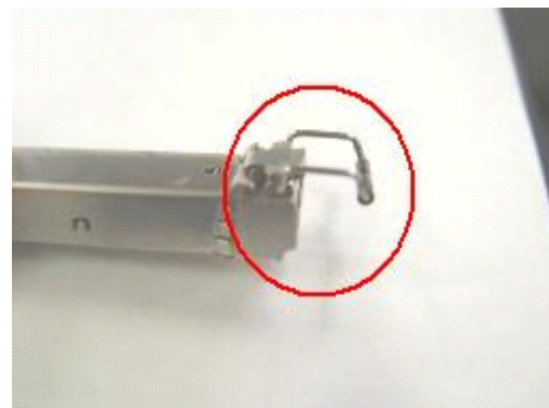
Open the release handle
