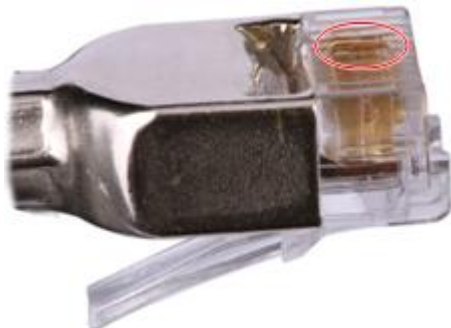
Figure 5-34 Unparallel contact strips of different heights
