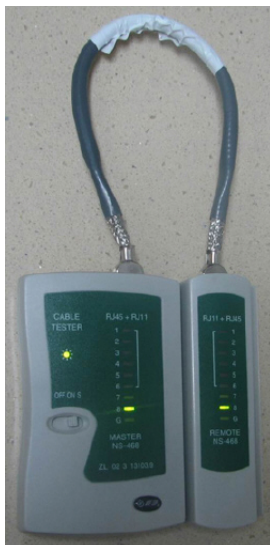
Figure 5-39 Testing the conduction and connections of wires
