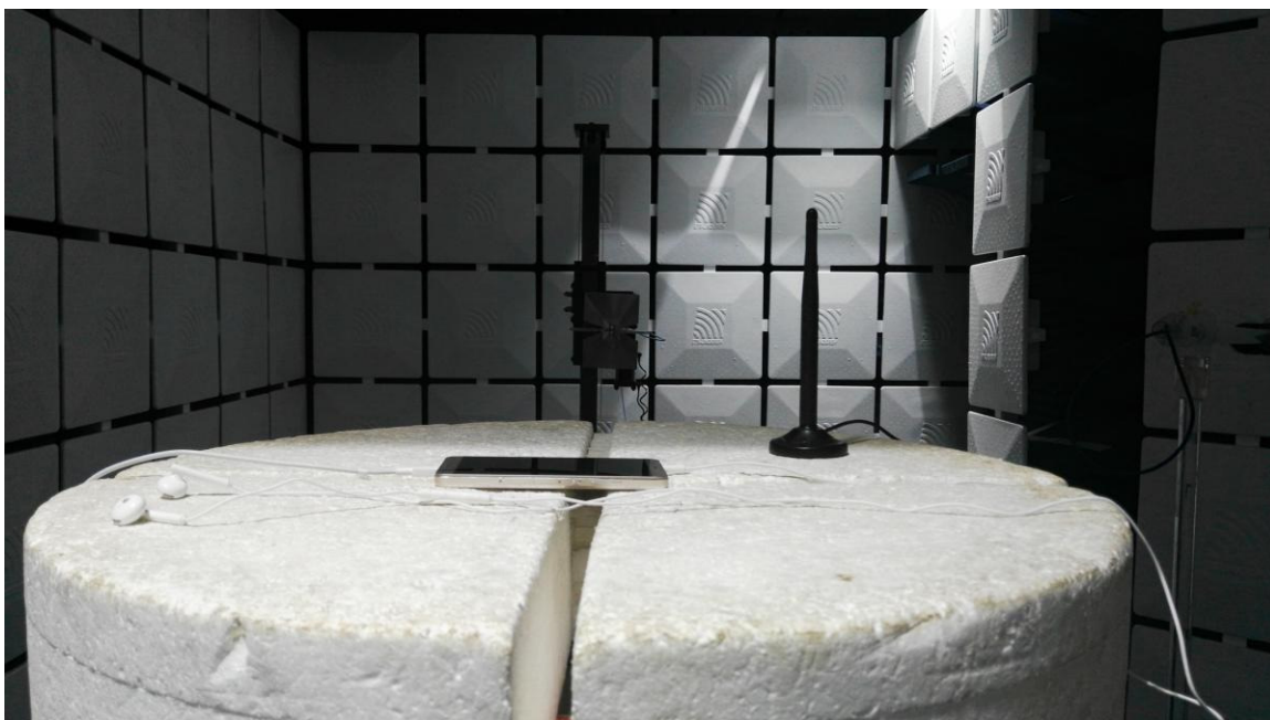
Radiated Spurious Emission (3GHz to18GHz)
