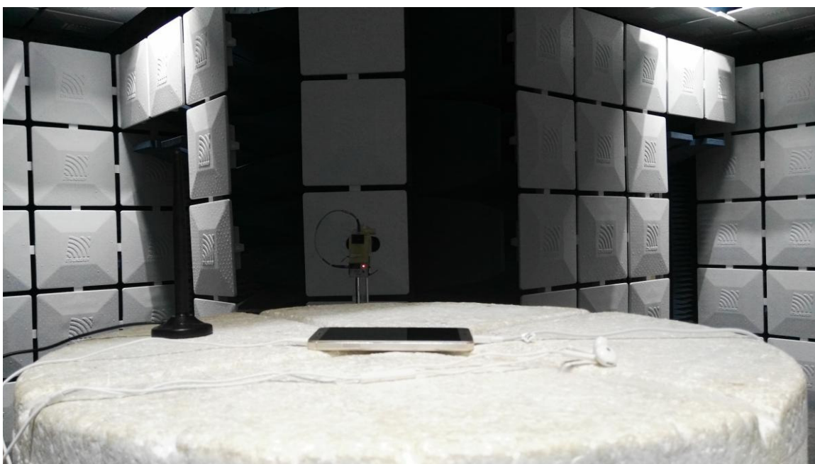
Radiated Spurious Emission (18GHz to26.5GHz)
