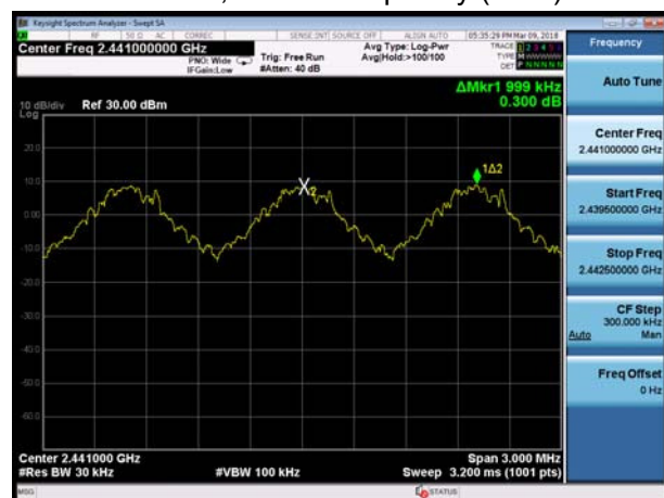
BT 3DH5 CH39, Carrier frequency (MHz): 2441
