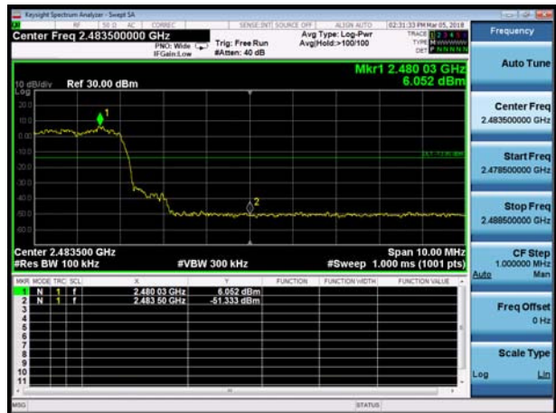
BT 3DH5 CH78, Carrier frequency (MHz): 2480
