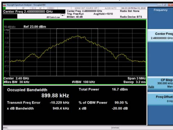
BT DH5 CH78, Carrier frequency (MHz): 2480
