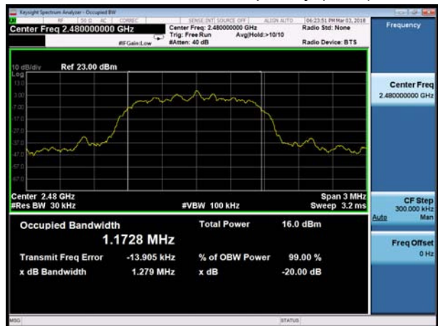
BT 2DH5 CH78, Carrier frequency (MHz): 2480
