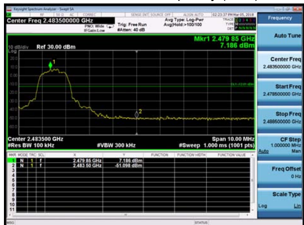
BT 3DH5 CH78, Carrier frequency (MHz): 2480
