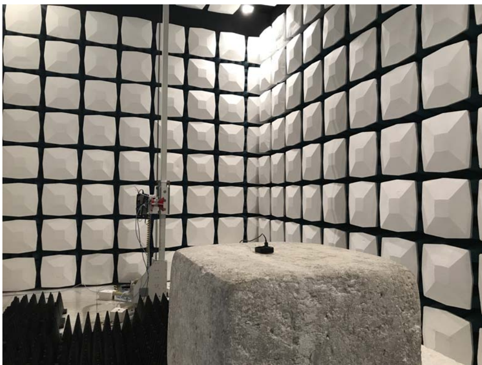
Description: Radiated Emission Test Setup for 1~18GHz
