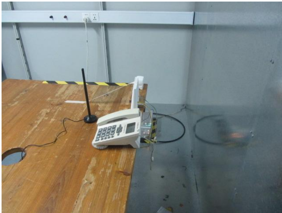
Conducted Emissions with AC Ports
