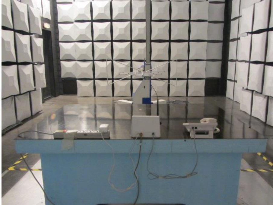
Radiated Disturbance Emissions (below 1GHz)
