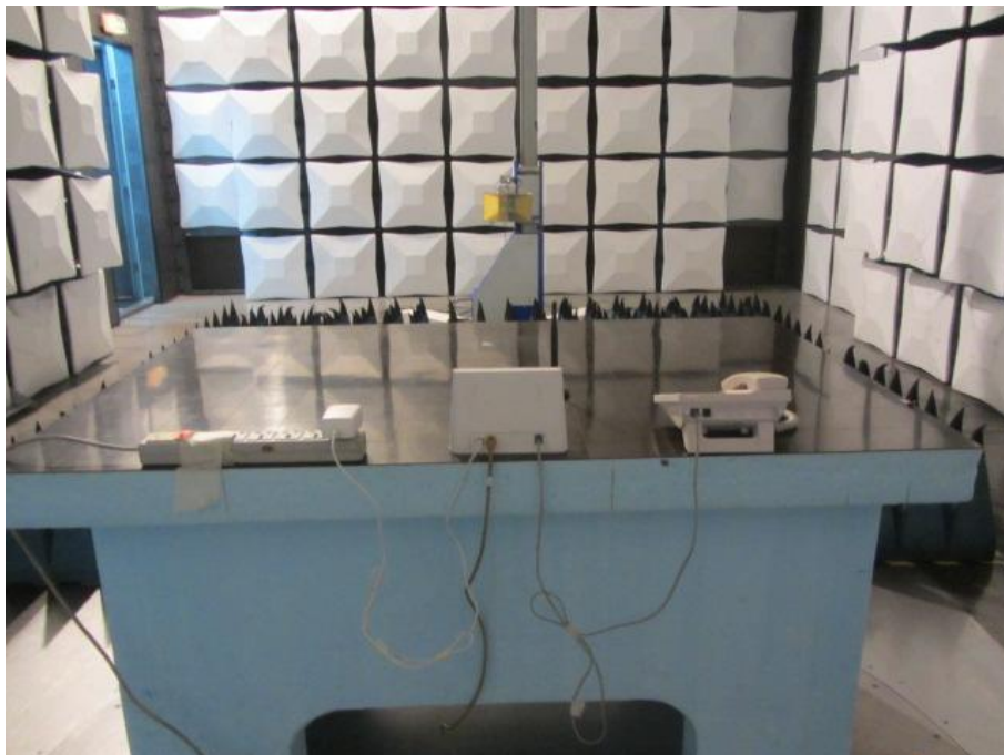
Radiated Disturbance Emissions (1GHz to18GHz)
