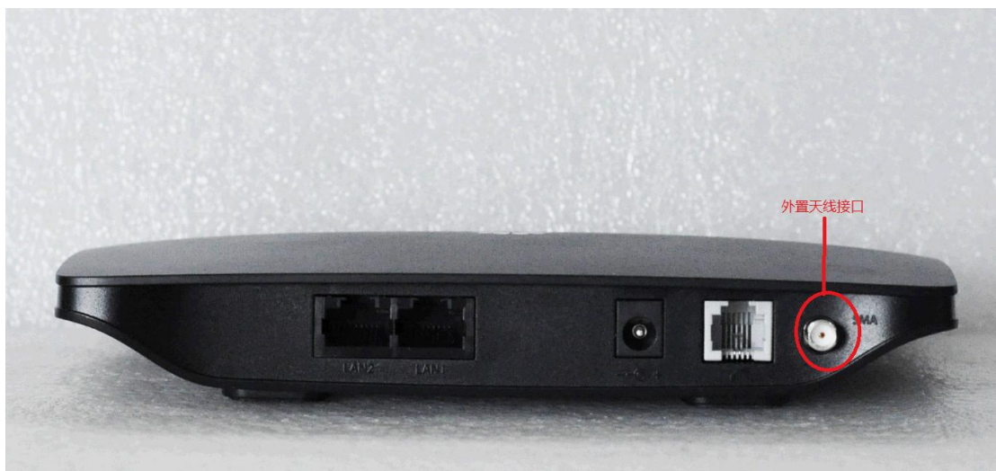
Picture 4(the external antenna interface on the B68L-54/B68L-25): The interface is not new added, it is already exist on the B68L-54/B68L-25.
