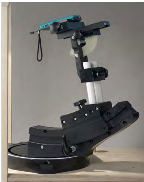
F-2. Device Holder for Transmitters
