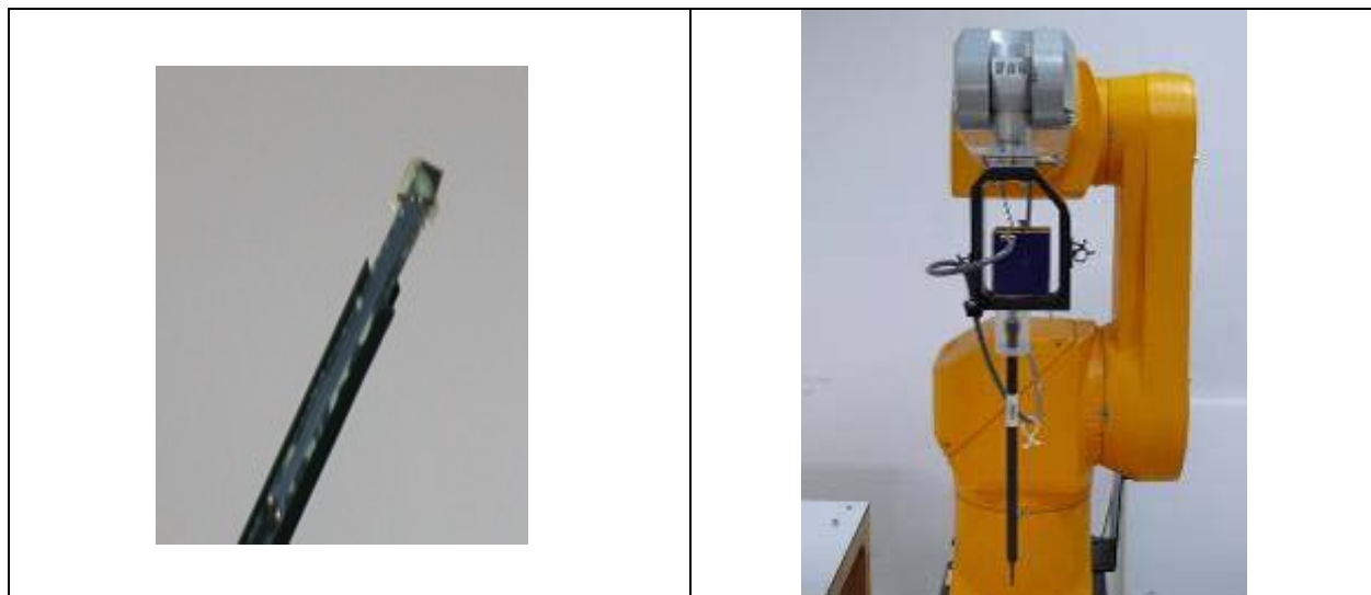
EX3DV4 E-field Probe
