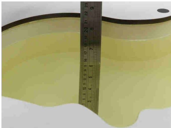
Fig 10.1 Photo of Liquid Height for Head SAR
