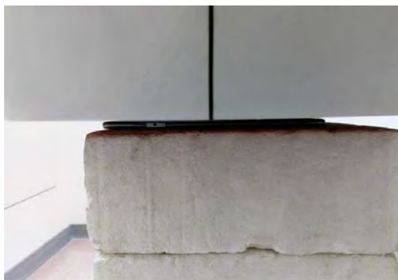
Fig.4 EUT Back side to flat phantom
