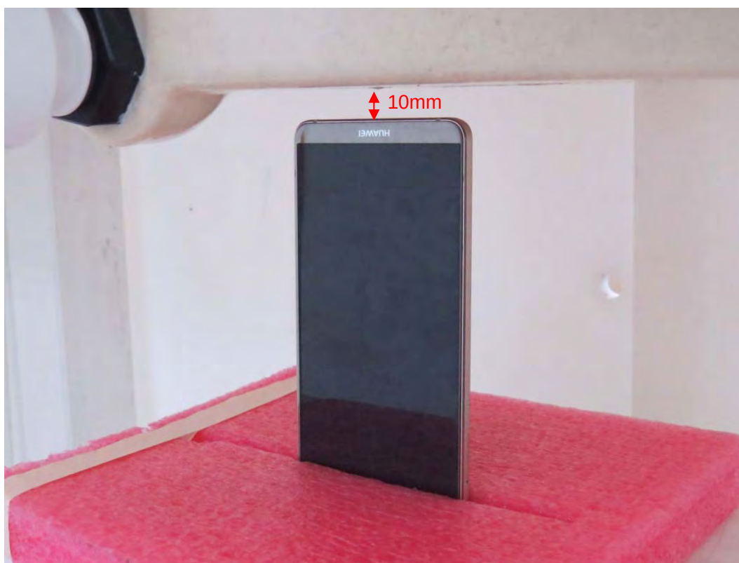
Picture 33: Bottom Side, the distance from handset to the bottom of the Phantom is 10mm
