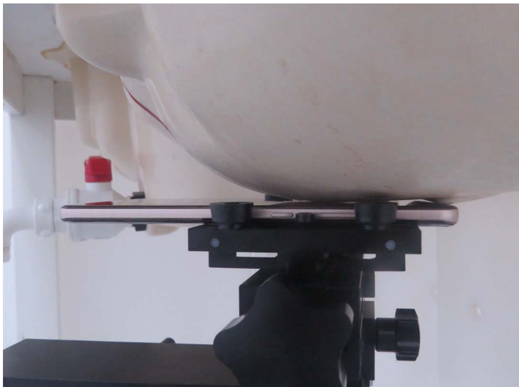
Picture 1: Left Hand Touch Cheek Position
