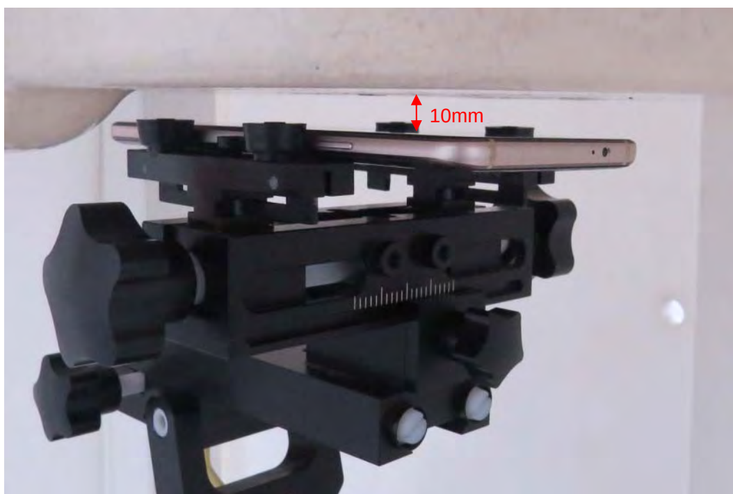
Picture 29: Front Side, the distance from handset to the bottom of the Phantom is 10mm
