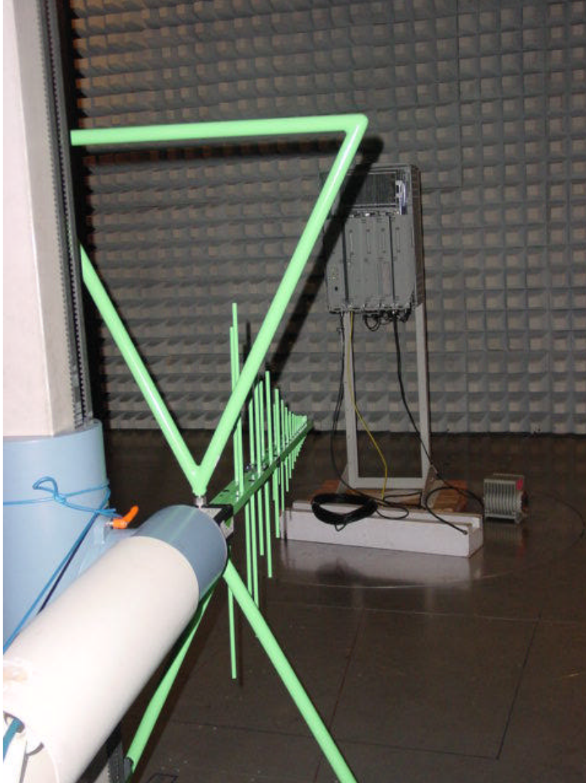
Photo ERP Measurement 30 MHz – 1 GHz
