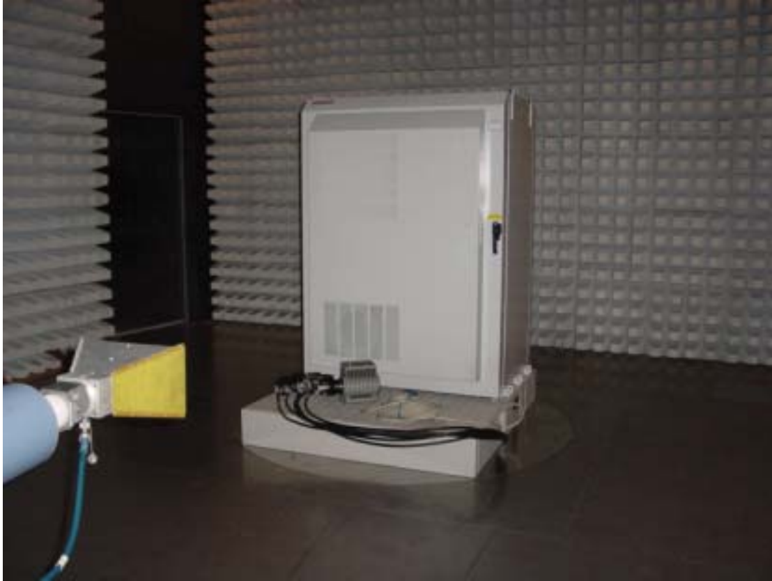
Photo ERP measurement 1 GHz – 10 GHz
