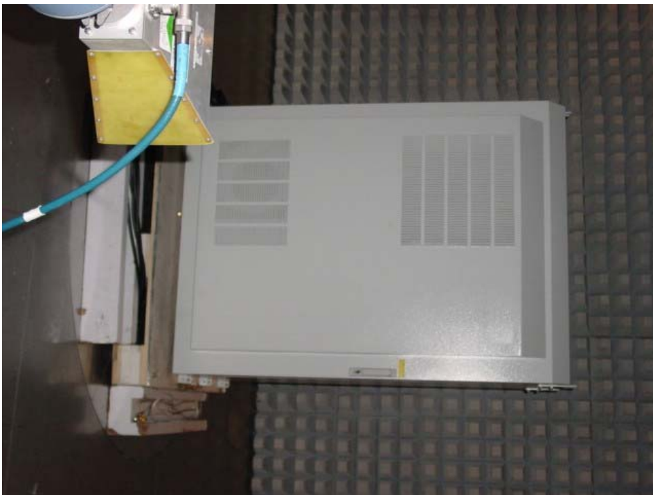
Photo ERP measurement 1 GHz – 10 GHz
