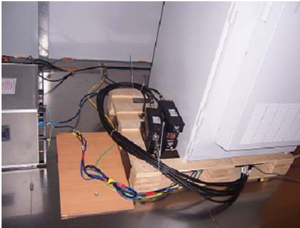
Conducted Disturbance at AC power port
