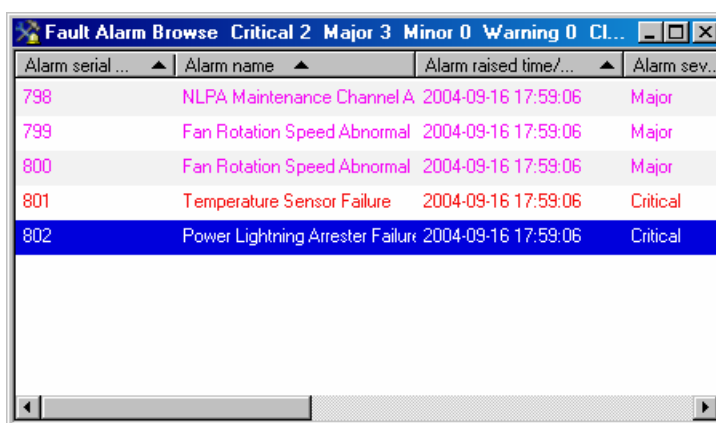
Figure 5-4 Fault Alarm Browse window
