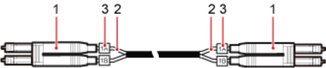
Figure 4-6 FE/GE fiber optic cable (2)
