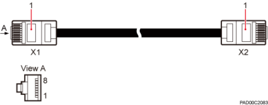
Figure 4-4 Appearance of an FE/GE Ethernet cable
