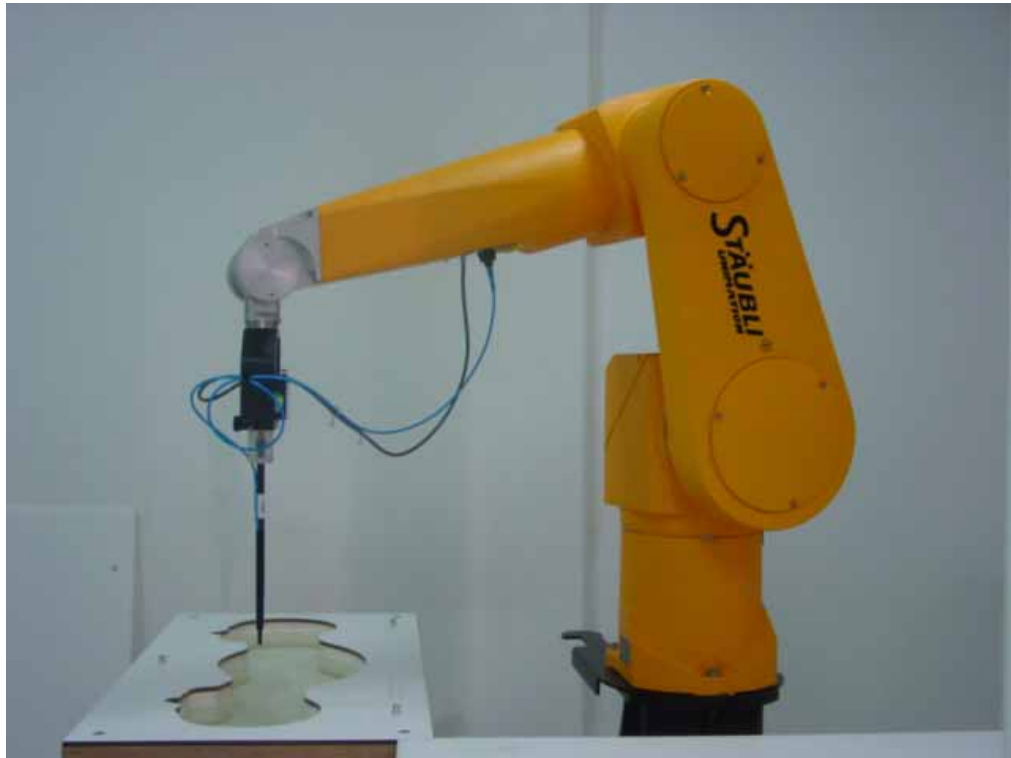
Picture 1 Specific Absorption Rate Test Layout
