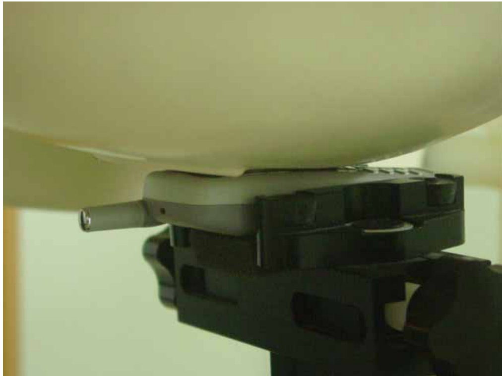
Picture 4 Right Hand Touch Cheek Position
