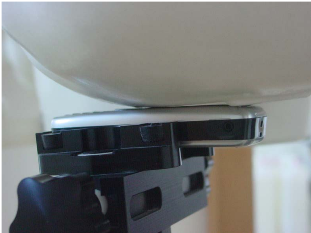
Picture B3: Left Hand Touch Cheek Position
