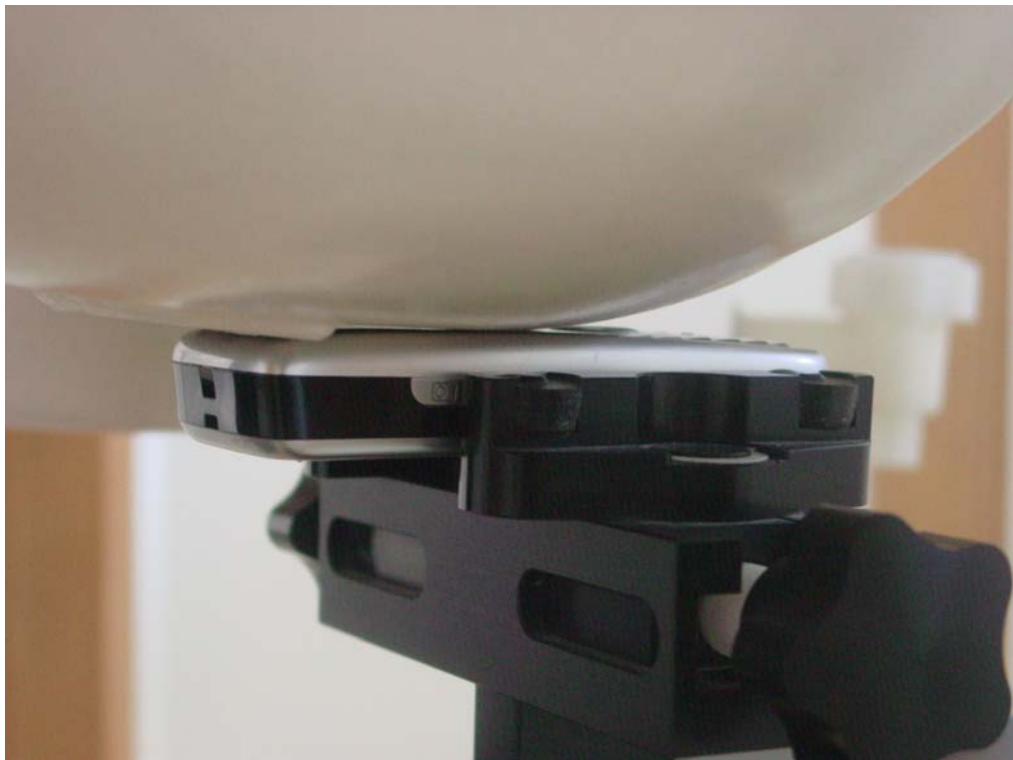
Picture B5: Right Hand Touch Cheek Position
