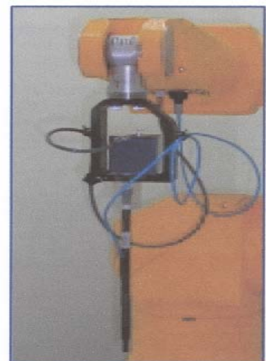
Picture4:ET3DV6 E-field probe
