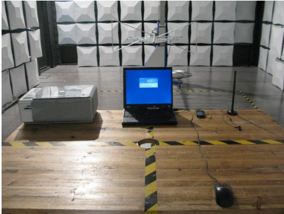
Radiated Disturbance (30MHz-1GHz)
