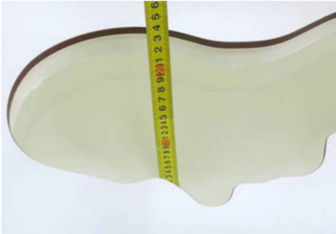
Picture 4: liquid depth in the head Phantom (2450 MHz, 15.2cm depth)
