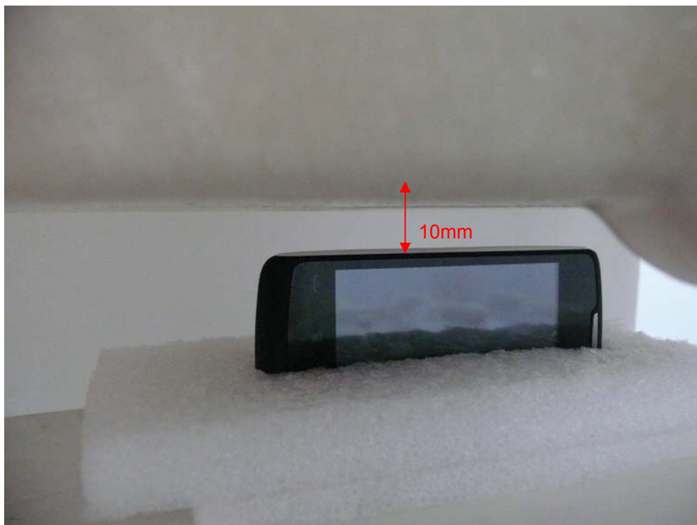
Picture 14: Left edge, the distance from handset to the bottom of the Phantom is 10mm
