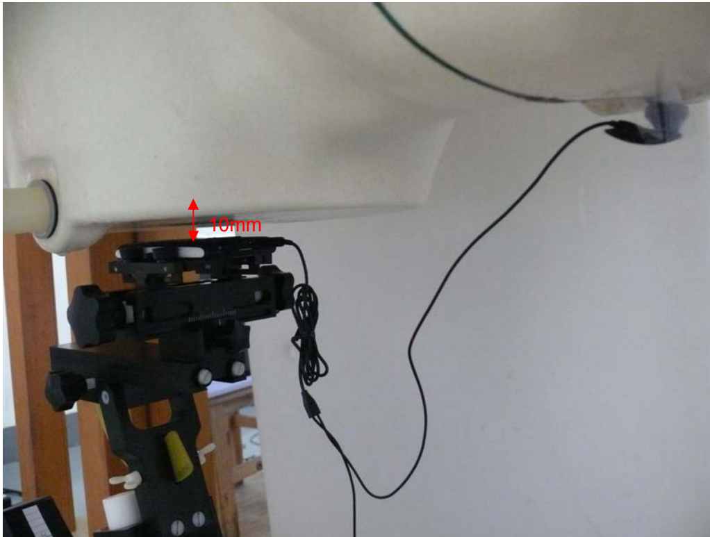
Picture 13: Body with Earphone, The EUT display Back Side, the distance from handset to the bottom of the Phantom is 10mm
