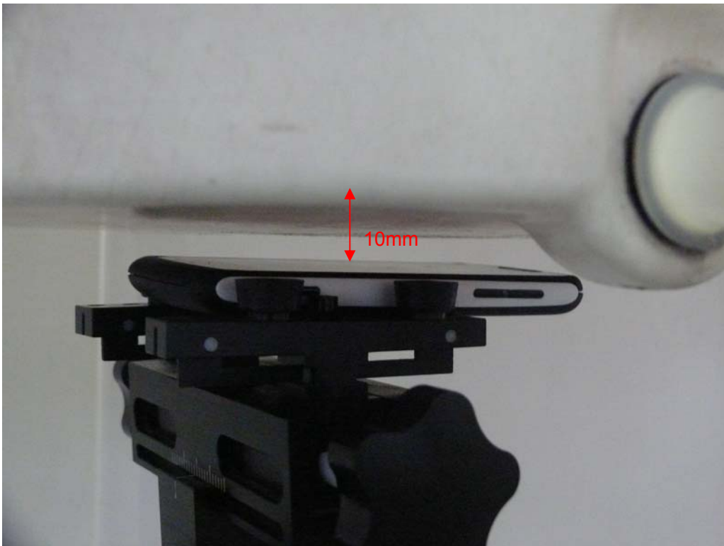
Picture 12: Body, The EUT display Front Side, the distance from handset to the bottom of the Phantom is 10mm
