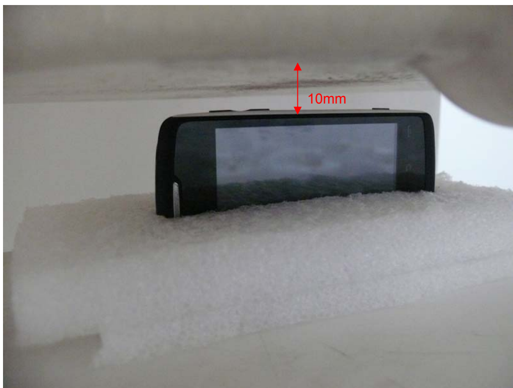
Picture 15: Right edge, the distance from handset to the bottom of the Phantom is 10mm
