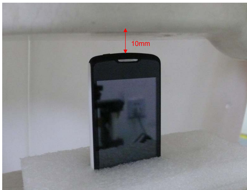
Picture 16: Top edge, the distance from handset to the bottom of the Phantom is 10mm
