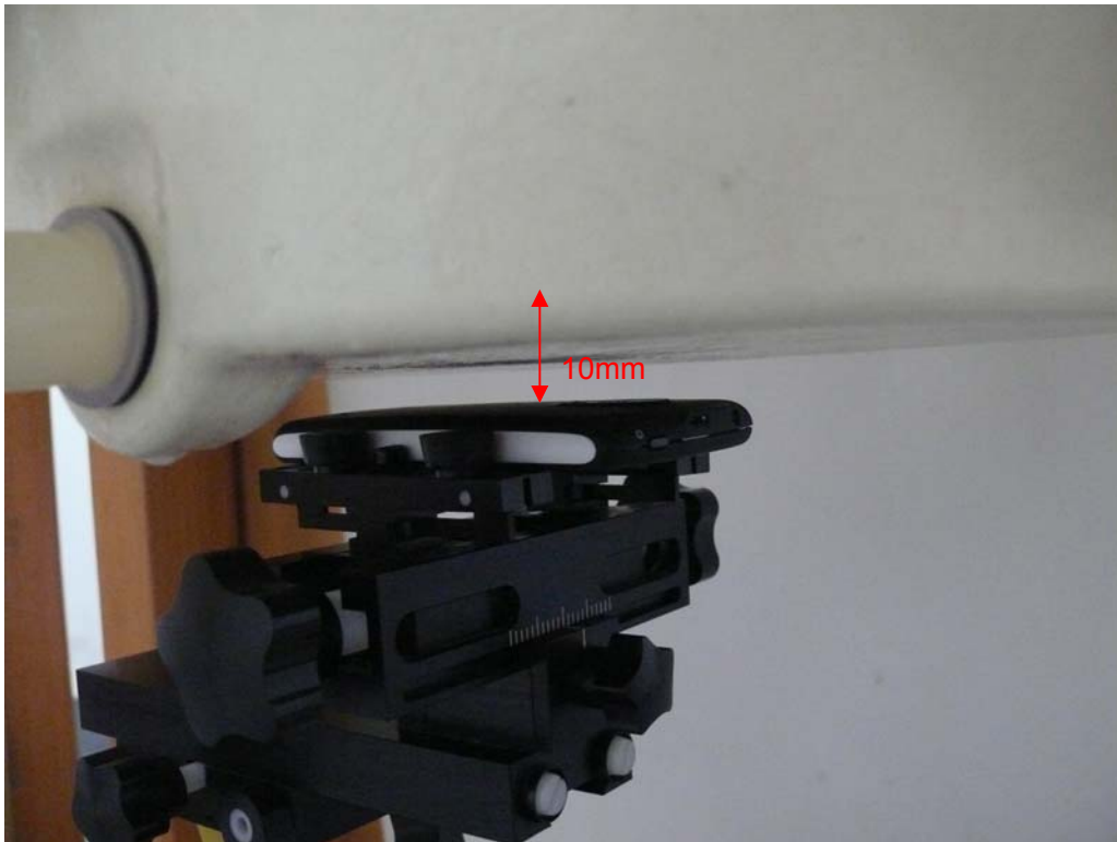
Picture 11: Body, The EUT display Back Side, the distance from handset to the bottom of the Phantom is 10mm
