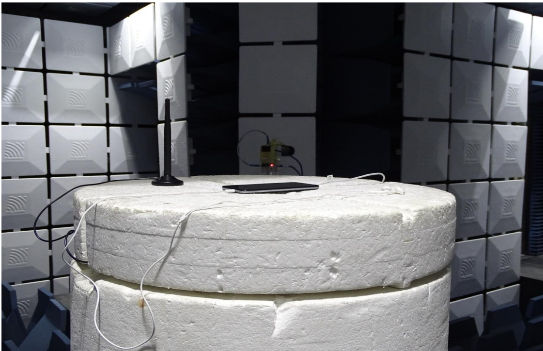
Radiated Spurious Emission (18GHz to26.5GHz)
