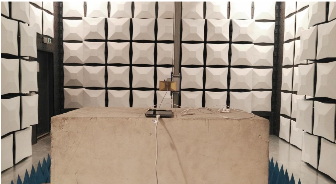
Radiated Spurious Emission (1GHz to 18GHz)
