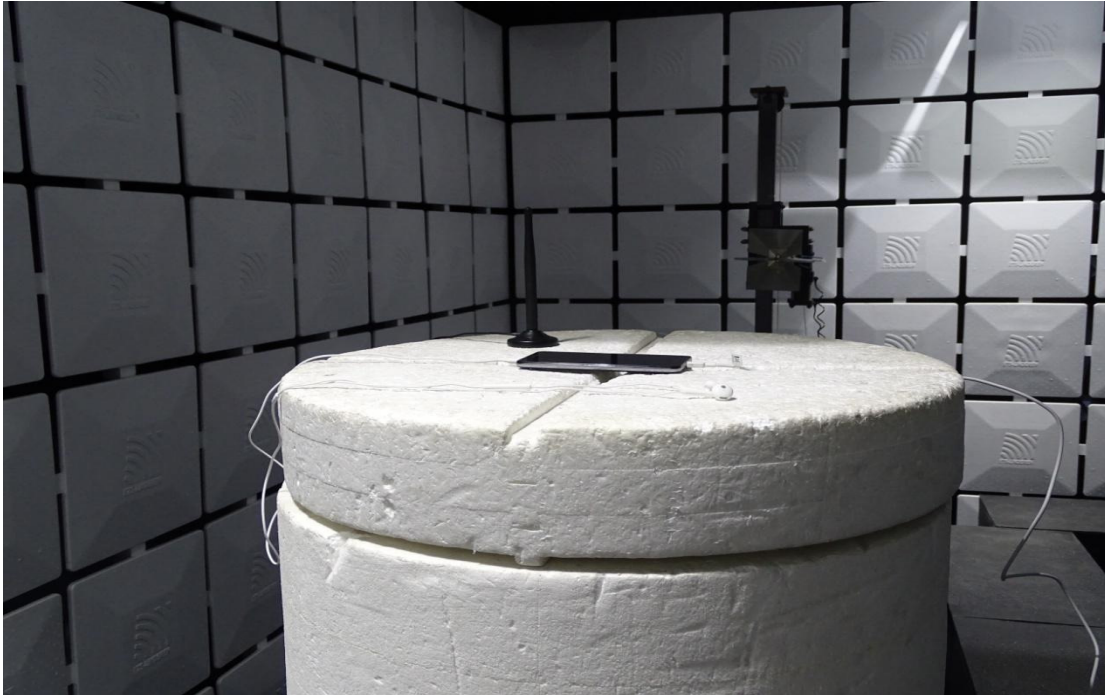
Radiated Spurious Emission (3GHz to18GHz)
