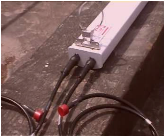
Figure 6-14 Appearance of the directional antenna after connection with jumper and connector processing
