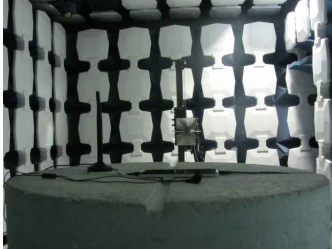
Radiated Spurious Emission (3GHz to 18GHz)
