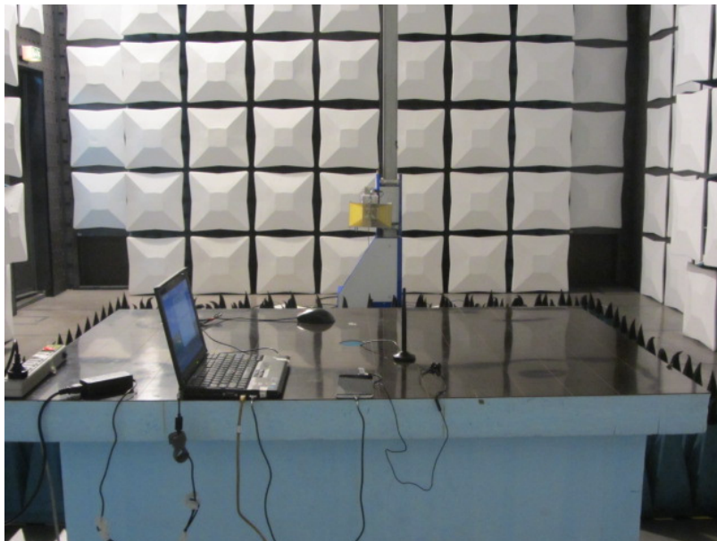
Radiated Spurious Emission (1GHz to 18GHz)
