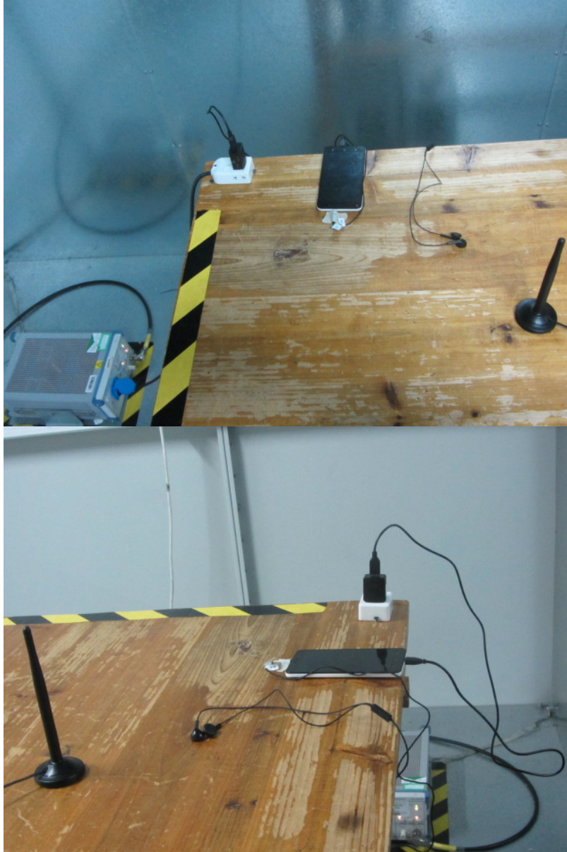
Conducted Emissions for AC Ports
