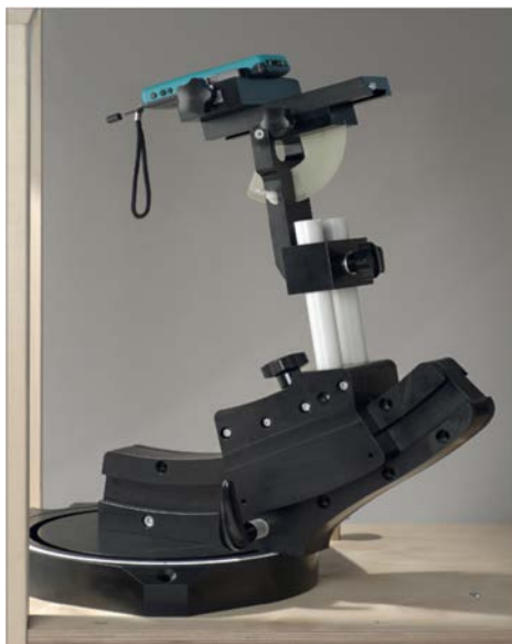
F-2. Device Holder for Transmitters
