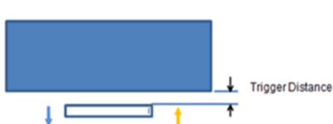
Picture: Proximity sensor triggering distances assesment for the back side
