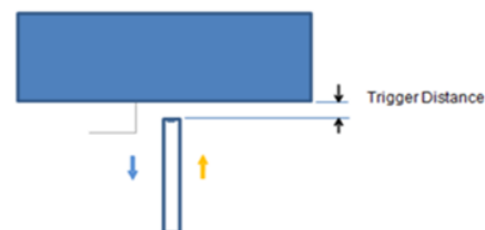
Picture: Proximity sensor triggering distances assesment for the Top side
