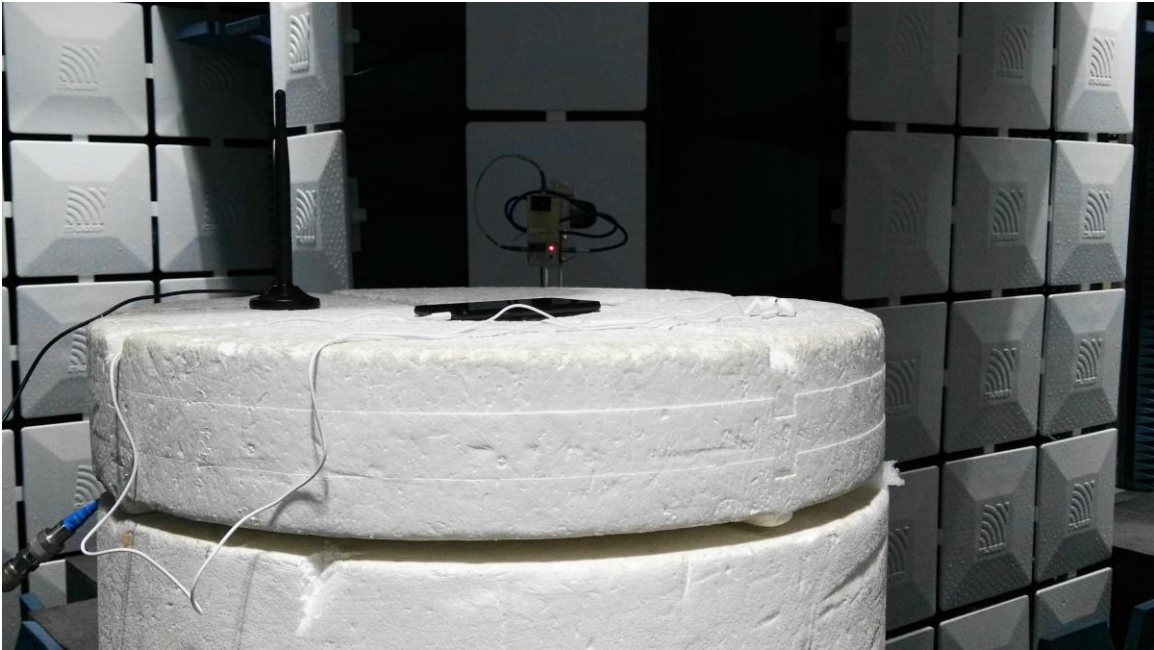
Radiated Spurious Emission (18GHz to26.5GHz)
