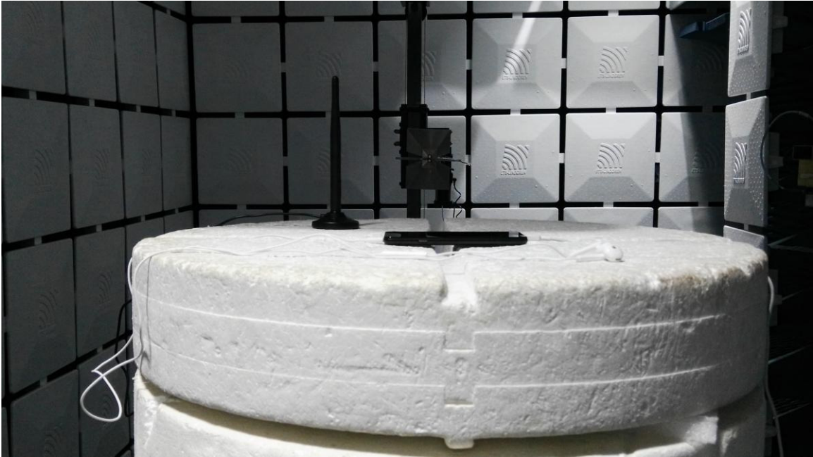
Radiated Spurious Emission (3GHz to18GHz)
