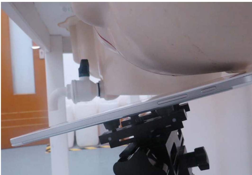
Picture 16: Left Hand Tilt 15 Degree Position
