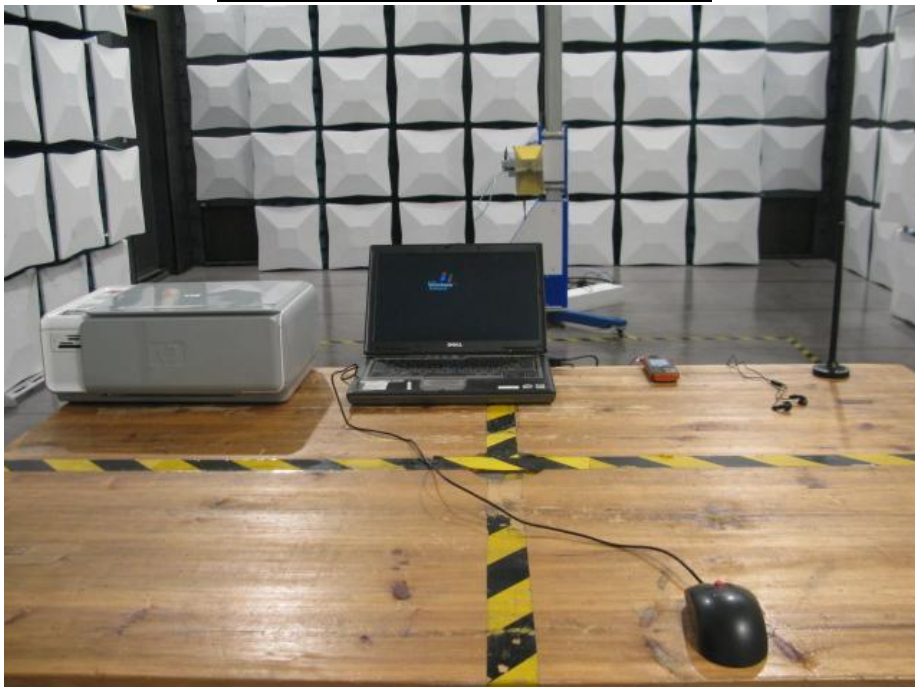
Radiated Disturbance (1GHz-18GHz)
