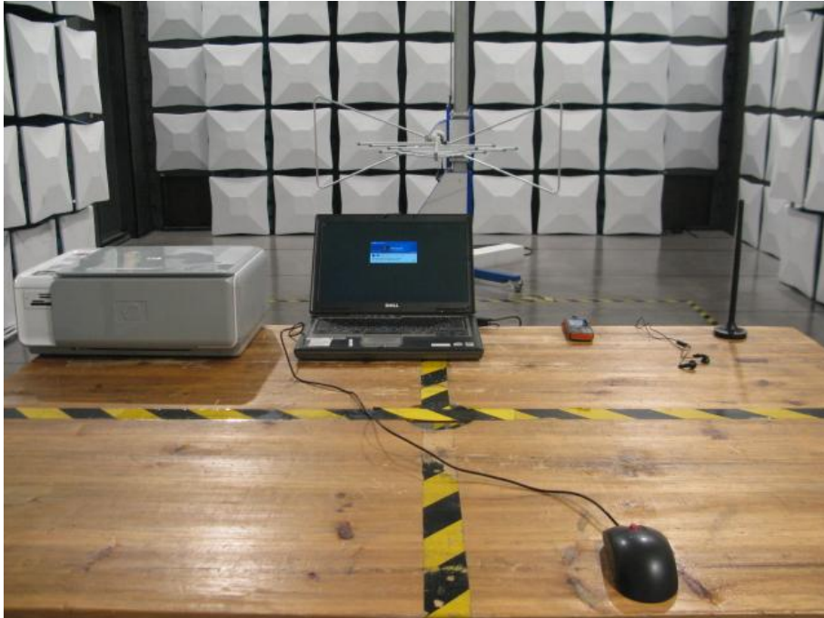
Radiated Disturbance (30MHz-1GHz)
