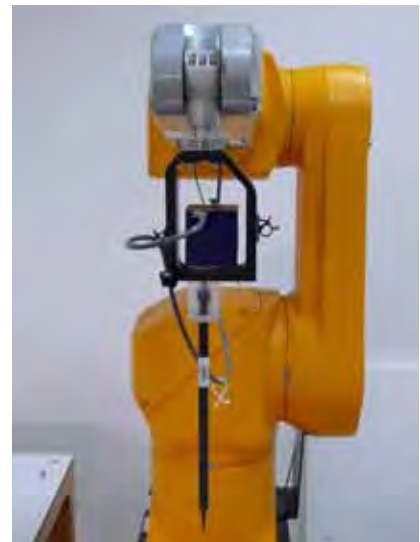
Figure 3. EX3DV4 E-field probe
