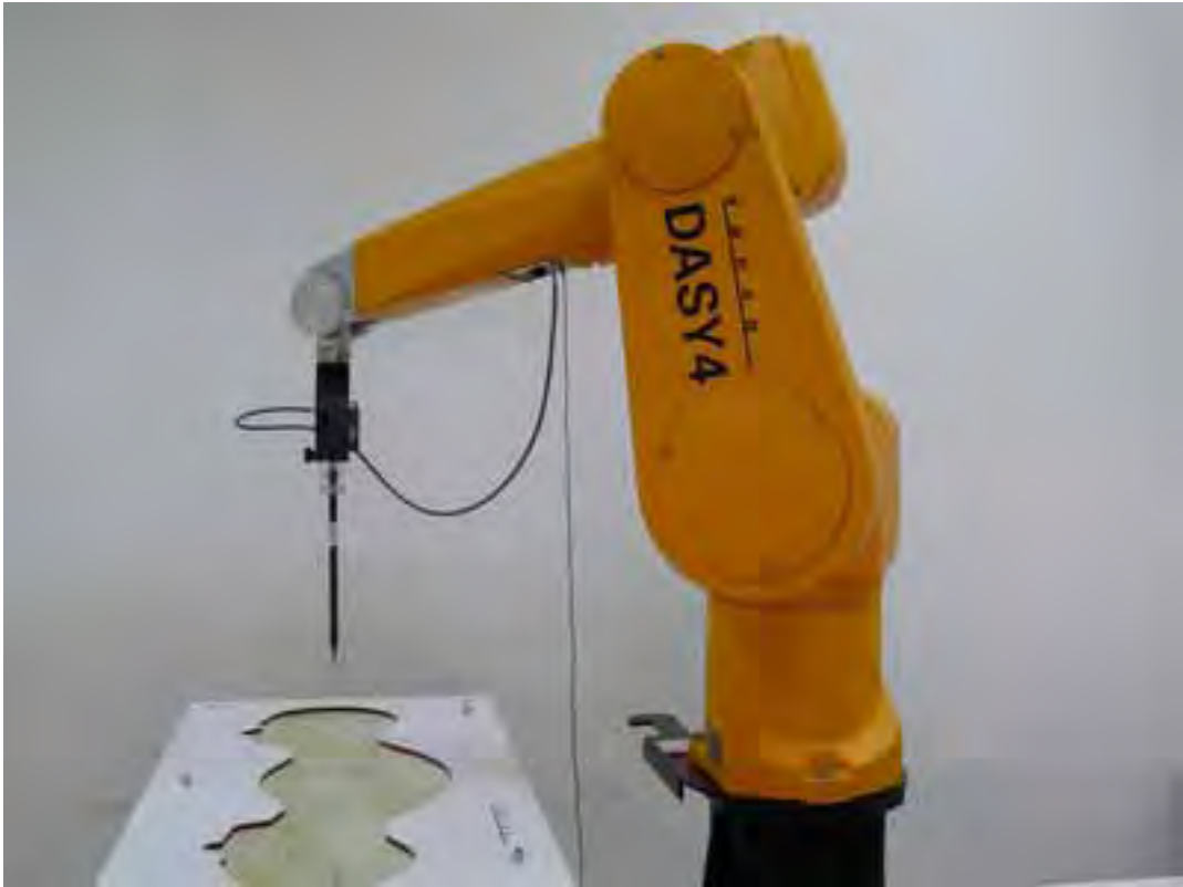
Picture 2 Specific Absorption Rate Test Layout
