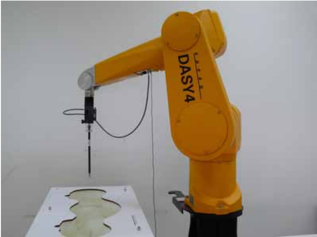
Picture 2 Specific Absorption Rate Test Layout
