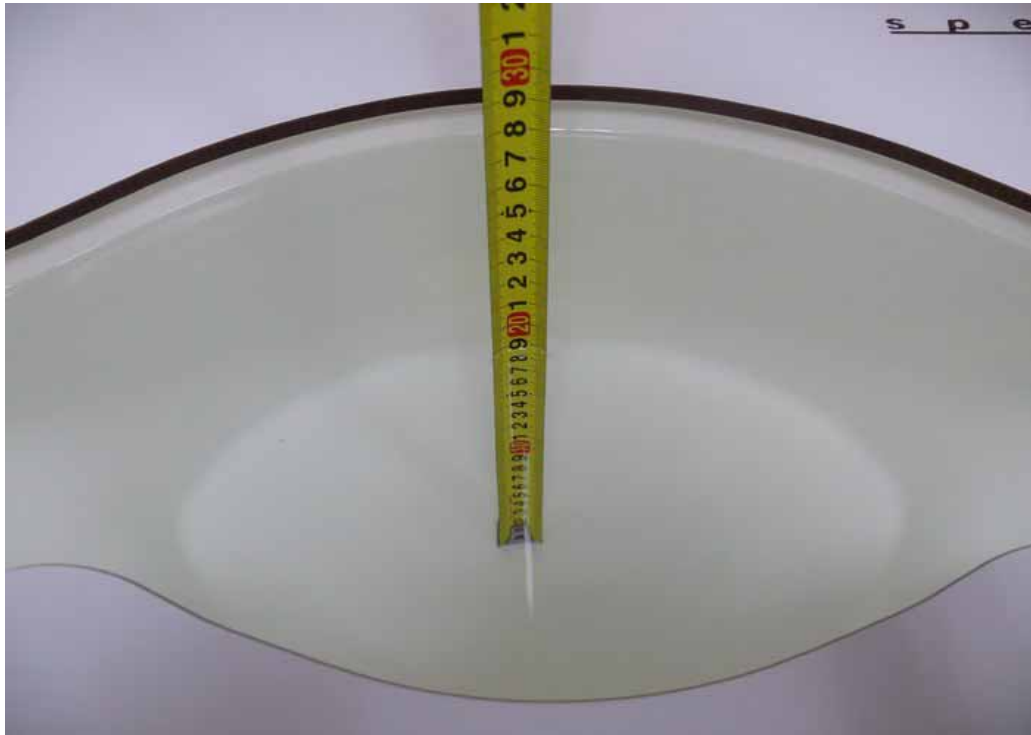
Picture 4 Liquid depth in the Flat Phantom (1900 MHz)
