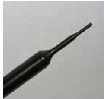
Figure 2. EX3DV4 E-field Probe
