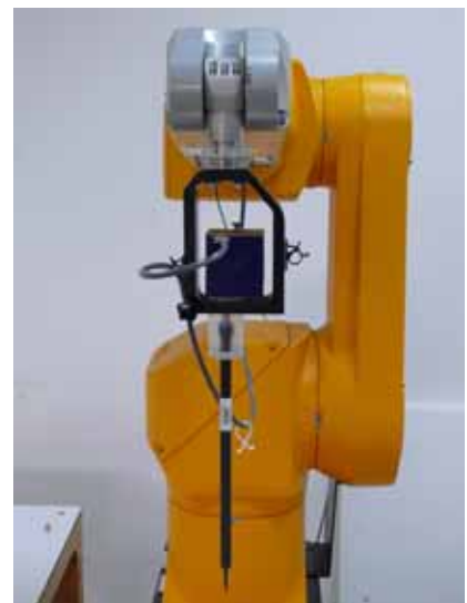
Figure 3. EX3DV4 E-field probe
