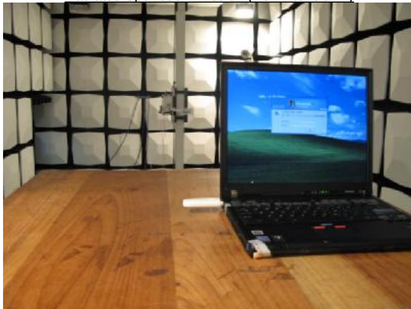
Radiated Spurious Emission 18G~26.5GHz
