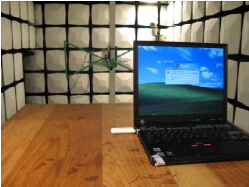
Radiated Spurious Emission (below 2GHz)
